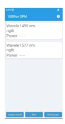
The 8 wavelengths at the bottom of the screen are calibration wavelengths, and selecting the corresponding wavelength can test the current optical power value. The test values are displayed in both dBm and nW units simultaneously. Clicking to stop the test program will stop the current test, and the data will remain displaying the last test result. Clicking to save the record will save the current test result.
