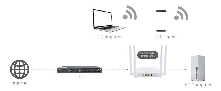
Figure: R52HD24XR Application Diagram
