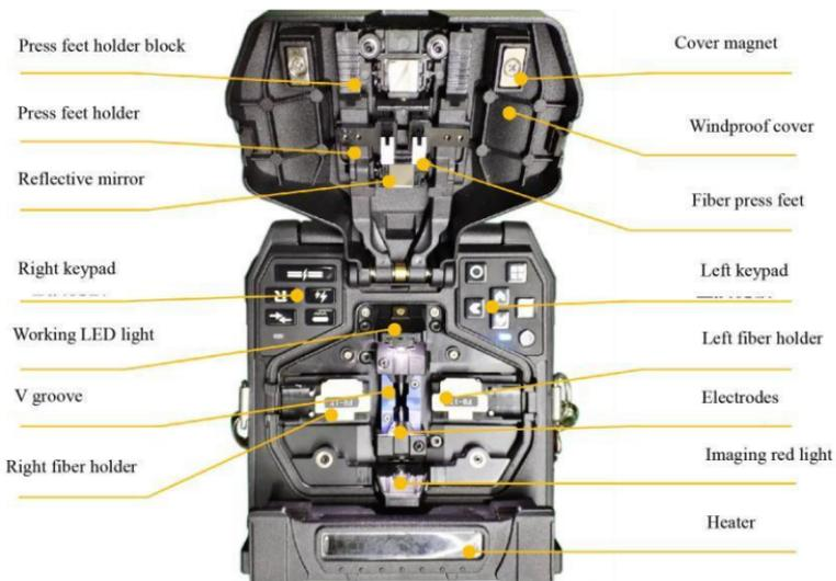
Figure 2.2 Main Structure Parts
