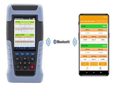
With the upgrade of GPON networks to XG(S)-PON, we have launched the new FOH-200XGS-BASE to apply for the installation and maintenance testing of the upgraded Combo PON network. By connecting FOH-200XGS-BASE to the PON network, we can quickly and accurately extract OLT information including OLT PON-ID, ODN class, Tx power, power level and ODN link loss pass/fail per ITU-T.
