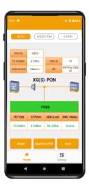
With the upgrade of GPON networks to XG(S)-PON, we have launched the new FOH-200XGS-PRO to apply for the installation and maintenance testing of the upgraded Combo PON network. By connecting FOH-200XGS-PRO in series to the PON network, we can quickly and accurately extract OLT and ONU information, support testing GPON and XG(S)-PON at the same time.
