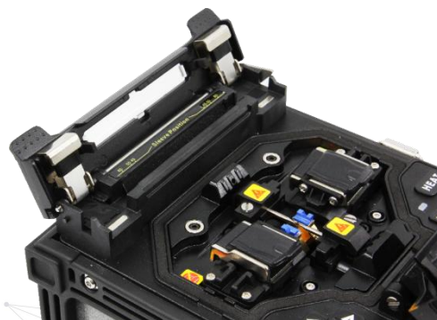
Inductive automatic heater (Heating time and temperature both adjustable)
