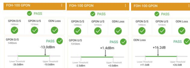
(4) Click "Threshold setting" to enter the PASS/FAIL qualification threshold setting for the downstream 1490nm and upstream 1310nm signal power level.
