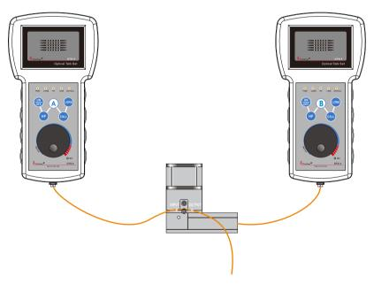
**Note:** The clip connection method showed above is just one model. The actual connection depends on the clip coupler you use.
