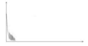
If the tested trace is just like the figure shows above, this might be caused by several reasons like: a bad connection between the connector and the lunching port, the optical pulse cannot be launched into the optical fiber or a short distance broken point of the tested fiber from the initial connection and the preset testing distance and pulse width is larger.
