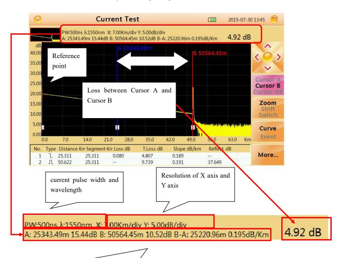
Indicate distance of cursor A and cursor B which relative to the reference point(start event), relative distance(km) and loss(dB) between cursor A and cursor B.
