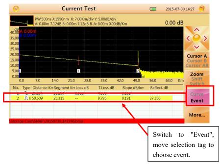
Every time move selection bar to an event in event list, cursor will move synchronously to relevant event on curve. User could use "Zoom", "Move", "Switch "function to adjust curve to a better position, for more information please read next sections.
