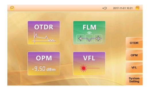
Select "FLM" module and press [OK] to enter FLM interface as below:
