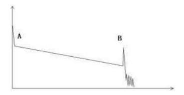
A normal trace shows as above, the A mark is a start-peak and the B mark is a end-reflection-peak. The tested trace is oblique, the total loss will become bigger with the increasing of the fiber length. The total loss(dB) divides total length is the average loss(dB/km) of a fiber.
