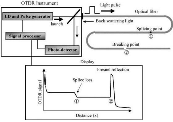
Working Principle of OTDR
