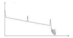
If there is additional reflection peak in a tested trace, this may be caused by a connection point or some other reasons. Anyway, appearance of the reflection peak shows that the two connecting surfaces of the connection are smooth. The smoother the connection surfaces are, the higher the reflection peak is.
