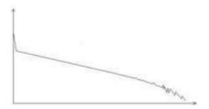
This situation often happened in a long distance testing, caused by under-range dynamic range of the OTDR that the energy of it can not support a long distance transmission or caused by a under-range preset testing range of distance or pulse width corresponding to the actual fiber length.
