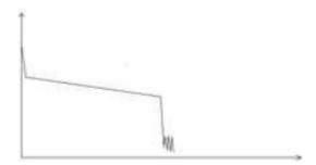
The situation that there is no reflection peak at the end of a trace shows above should be paid attention on. If the distance of the tested fiber is available and the distance shown on OTDR is not equal to the original distance, this shows that the fiber might be broken down or twisted and the bending radius of it is over limited. The distance shown on OTDR is the position of the fault point.
