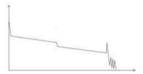
There is a common phenomenon that an obvious step is on the middle of a tested trace, it often caused by a fiber bending, fiber knot, being pressed by something heavy or a fuse splicing point. The step means a bigger loss of a fiber, it is also called event point. If the direction of it is downward, it could be called non-reflection event. If the direction is upward, we can call it reflection event.
