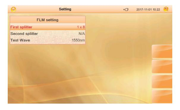
Press 【▲】 or 【▼】 to set "First splitter", "Second splitter" or "Test wavelength" option according to the actual condition of your fiber under test.
